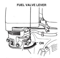
Figure 10. Fuel Shut-OFF Lever
